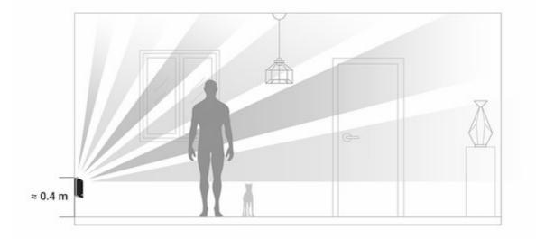
The placement of a MotionProtect Curtain also depends on the distance to a hub and whether there are any obstacles between the devices that may hinder the radio signal, e.g., walls, floor deck, or large objects in the room.
